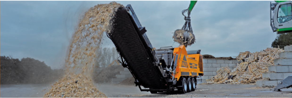
Grinding of waste wood/pallets
