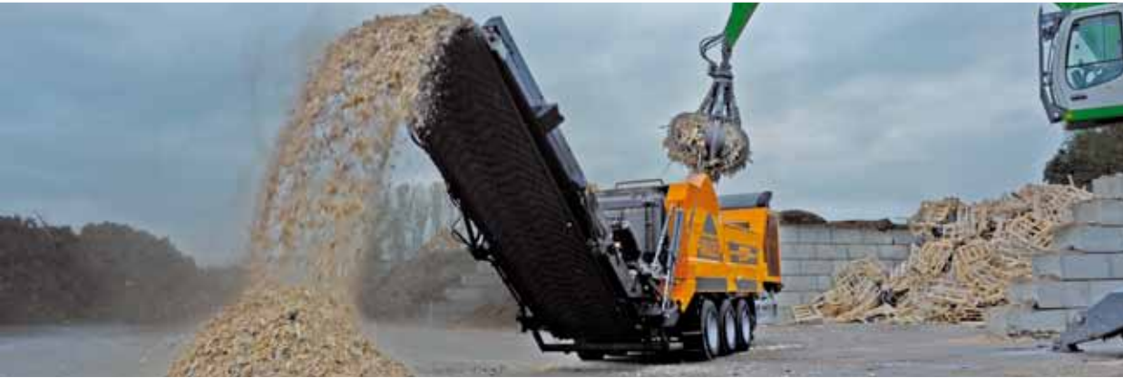
Grinding of waste wood / pallets
