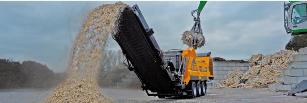
Grinding of waste wood / pallets
